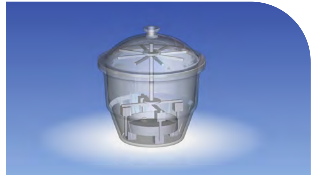
Figure 5. Representation of a flowers of sulfur test chamber
