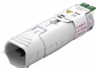
This module is designed for the surface treatment of non-conductive substrates such as plastics, ceramics or glass. For effective treatment, a module-substrate-distance of 1 to 5 mm is recommended. If uncontrolled arcing occurs on the substrate during use, the device switches off automatically. In this case the surface is at least partially conductive and should therefore be treated with the Nearfield module.
