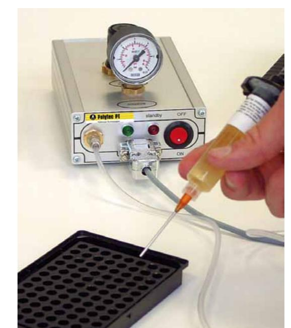
These dispensers are widely used in industry. They are low cost and accurate and may be used just manually or integrated in automatic systems. In general the adhesive is supplied in cartridges. So, the user just has to put the cartridge in his dispenser and begin dispensing. The procedure is really failsafe.
