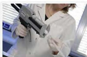
4. Good quality mixing is key to a successful bonding operation. The recommended mixing nozzle is attached to the cartridge.
