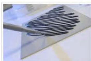
6. A thin bead of adhesive can be easily applied direct from the mixing nozzle.
