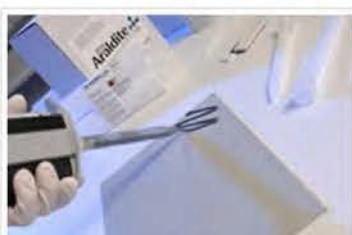
5. The first drops of adhesive should be discarded, to ensure that both hardener and resin are flowing through the mixing nozzle in correct proportion.
