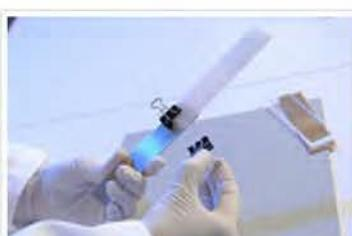
11. The parts are then clamped in order to retain a certain pressure until the adhesive has reached handling strength.
