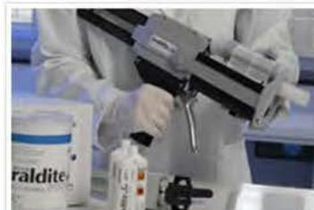
3. For each cartridge size, an appropriate dispensing gun is used. In this case, the adhesive is supplied in a 200ml cartridge.
