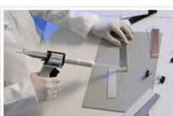
8. A small bead of adhesive is applied onto the substrates to be bonded.
