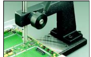
Figure 3: Eyelets can be set in place using an Eyelet Press.
