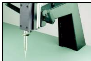
Figure 4: Bond the new BGA pad with a Bonding Iron or Circuit Bonding System.
