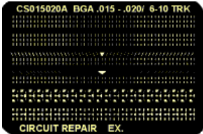
Figure 2: Select a replacement BGA pad that matches the missing pad.
