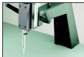
Figure 3: Bond the lifted conductor using a Bonding Iron or Circuit Bonding System.
