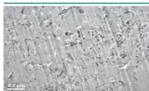
■ ARE-310 MWNT is uniformly dispersed in 2-part thermosetting resin.
