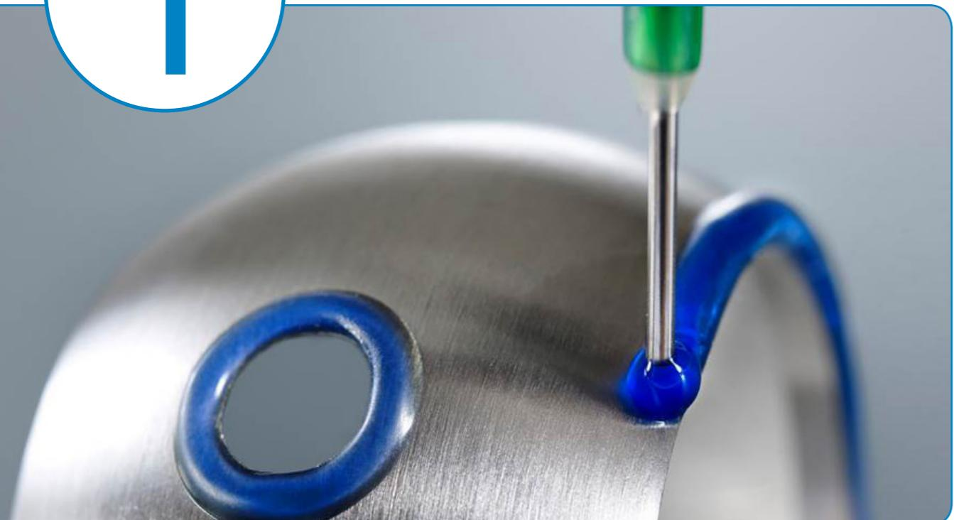
SpeedMask® can be easily applied and provides numerous masking possibilities - even for complex components. The dimensionally stable characteristics make the masking of cavities or holes and the application on horizontal or vertical surfaces a lot easier.
