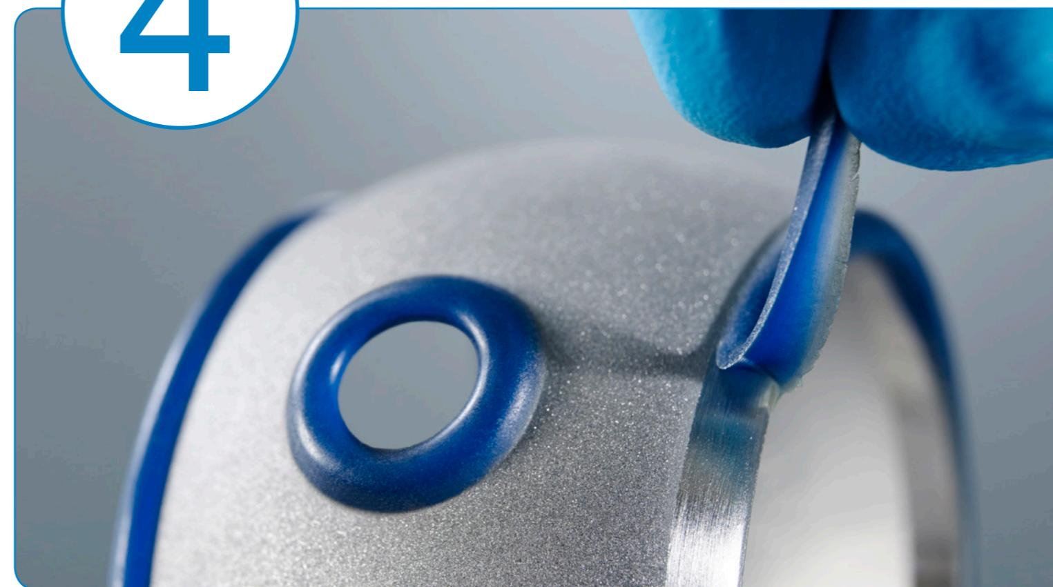
Immediately after the surface processing is finished, the temporary mask can be removed. There are a couple of ways to accomplish that:
