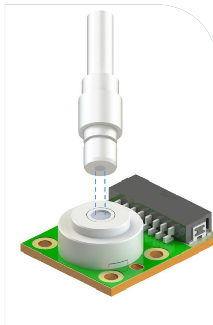
Figure 11. Aperture with 3-mm Lightguide
