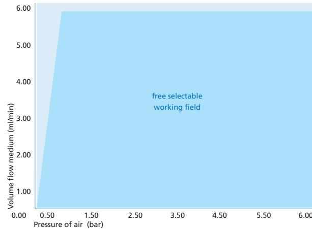
Working field is free selectable. Volume flow of air & medium are independently adjustable.
