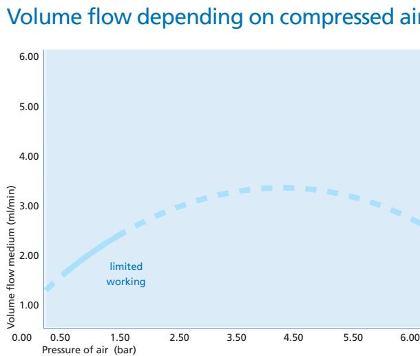
Limited working field. Volume flow of air & medium are interdependent.
