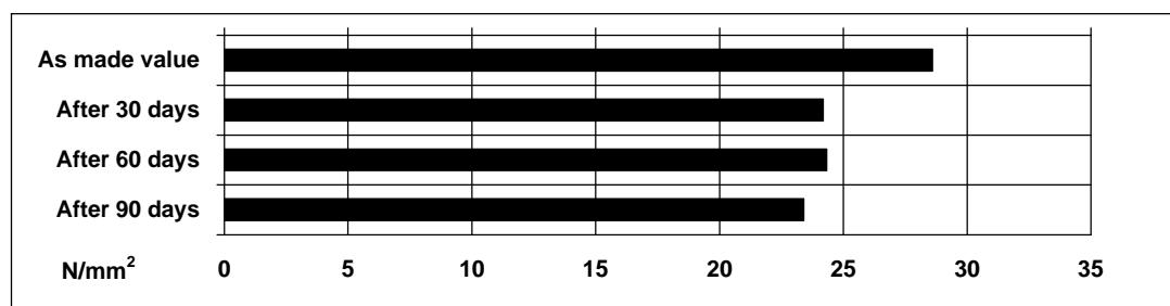
**Lap shear strength versus heat ageing 70°C for 30, 60 and 90 days.** Typical average value on aluminium
