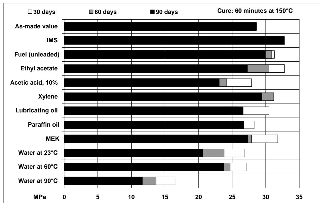
**Lap shear strength versus tropical weathering** (40/92, DIN 50015; typical average values on aluminium)
