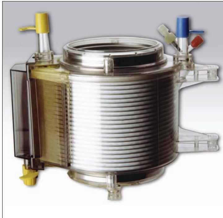
An LCM gives designers a 100% seal between the cap and the polycarbonate housing of an oxygenator. The housing passes the assembly point where the LCM is applied, the cap is slid over it, and UV light cures the adhesive in seconds.
